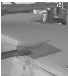
The alveolar core is setup on the mould
